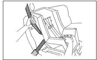
5. To tighten the belt, push down on the child restraint, pull the shoulder portion of the belt to tighten the lap portion of the belt, and feed the shoulder belt back into the retractor. If you are using a forward-facing child restraint, you may find it helpful to use your knee to push down on the child restraint as you tighten the belt.
